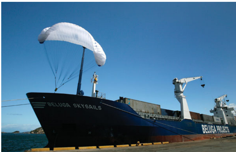
FIGURE 16.1 Wind power is becoming so popular that it is even making a comeback as a way to propel ships. Here a new kind of sail, actually a cable-tethered kite, helps pull a new ship, the Beluga SkySails , through the ocean. (Source: SkySails website March 31, 2008. First retrofit SkySails-System aboard a cargo vessel—Initial operation successful SkySails pilot project on board the MS “Michael A.” of the WESSELS Reederei GmbH & Co.KG based in Haren/Ems http://www.skysails.info/index.php?id=64&L=1&tx_ttnews[tt_news]=98&tx_ttnews[backPid]=6&cHash=c1a209e350 and http://www.skysails.info/index.php?id=64&L=1&tx_ttnews[tt_news]=104&tx_ttnews[backPid]=6&cHash=db100ad2b6 )
