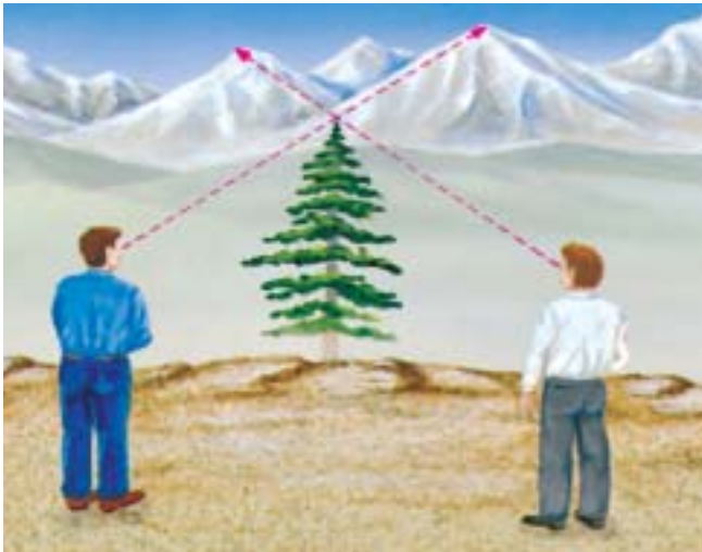
FIGURE 2-5 Parallax Nearby objects are viewed at different angles from different places. These objects also appear to be in a different place with respect to more distant objects when viewed at the same time by observers located at different positions. Both effects are called parallax, and they are used by astronomers, surveyors, and sailors to determine distances.
